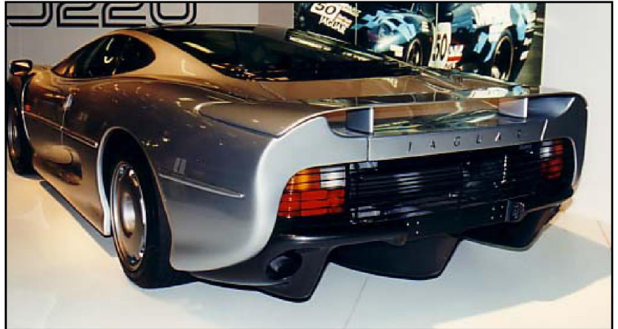
Above: Jaguar diffuser rear under-tray. The Ferrari Modena also utilizes this aerodynamic aide to cheat the wind. The Guara doesn't, it would be useful but this is still not a shame.
